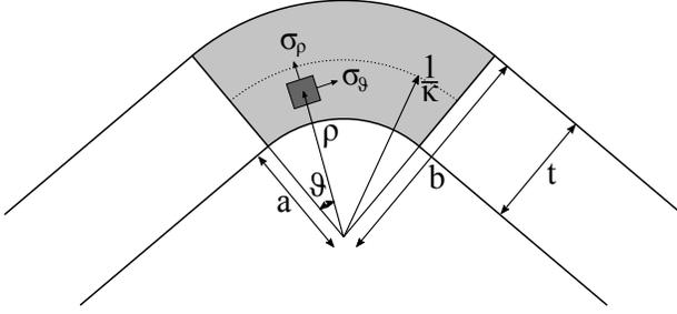
**Figure 2:** Geometry of the thick fold model in addition to the geometry defined in Fig. 1, which applies along the neutral axis (shown dotted).
