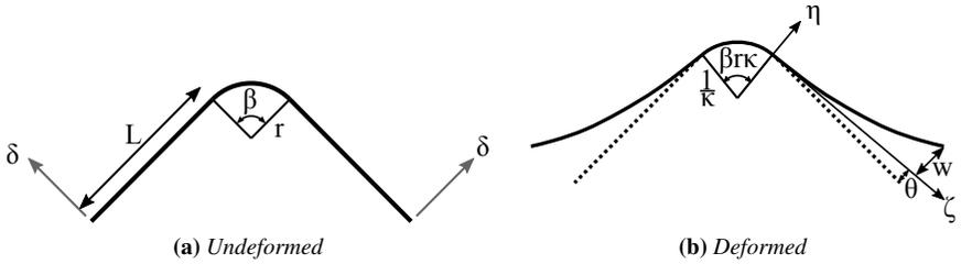
**Figure 4:** Cross-section geometry for a folded strip with deformable panels in the undeformed (a) and deformed (b) states. A displacement of  $\delta = w + L \sin \theta$  is imposed perpendicular to the panel which opens the strip by a combination of panel bending and fold opening.
