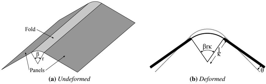
**Figure 1:** Fold cross-section geometry in the undeformed (a) and deformed (b) states. The panels are considered as rigid plates; therefore only the fold region deforms.
