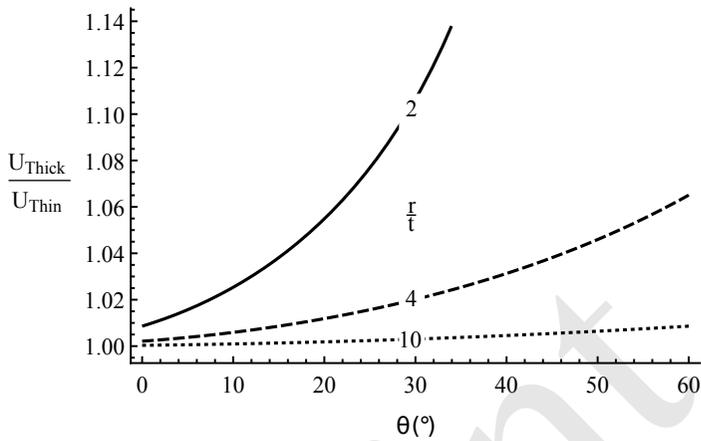
**Figure 3:** Ratio of thick and thin fold strain energies, Eqn 9 and Eqn 2, for a fold with  $\beta = 30^\circ$  and  $r/t$  ratios of 2, 4, and 10. For small values of  $r/t$  the thick fold model requires more energy to deform (it is stiffer). As the  $r/t$  ratio increases, the energy ratio approaches unity.
